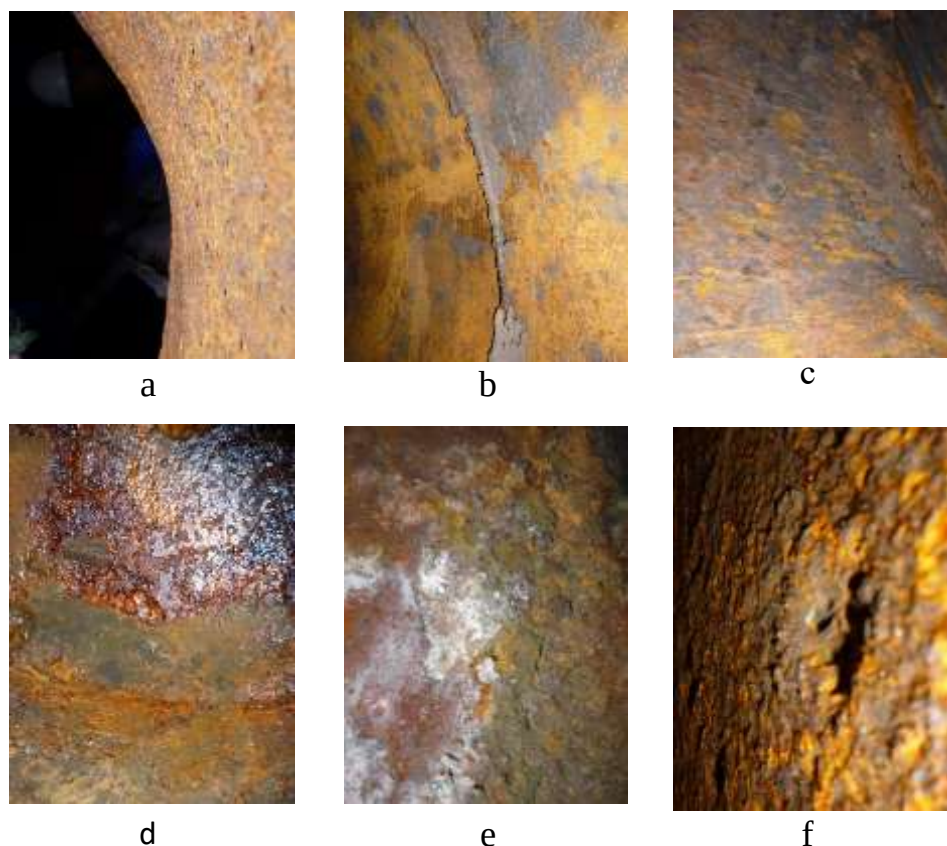
a) upper part (5-6 zones), b) middle part (3-4 zones), c) lower part (1.2 zones), d) bottom of the tank, e) uneven corrosion of the tank surface, f) destruction of the tank surface in the process corrosion.
