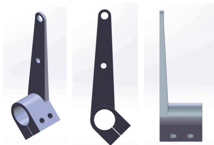
1-rasm. STB to'quv mashinasining zarb mexanizmi xaydagich richagi.
