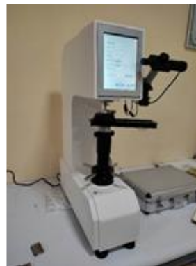
4-rasm. THBRV-187.5DX universal qattiqlikni o'lchash mashinasi
