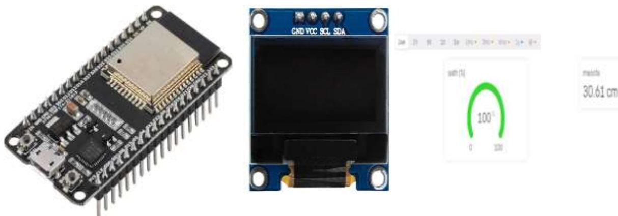
1-rasm: ESP32 radio moduli va SSD1306 OLED display.
