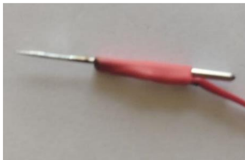
A) B) 1-rasm. Iгна haroratini o'lchash uchun termodachchik va uni ignaga o'rnatish.
