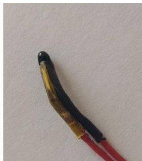
A) B) 1-rasm. Iгна haroratini o'lchash uchun termodachchik va uni ignaga o'rnatish.
