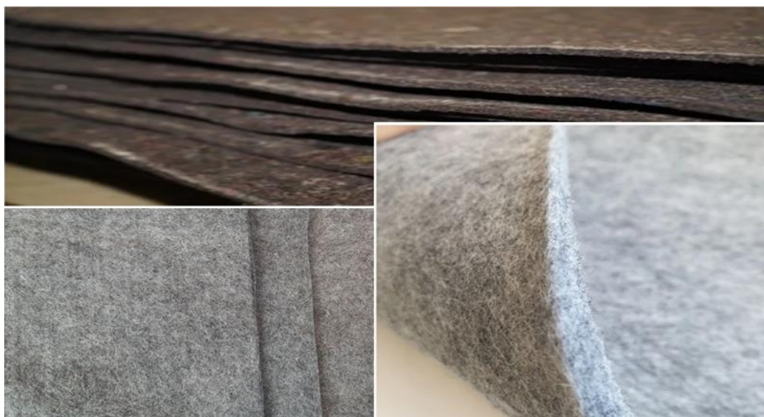
1-rasm. Jun tolalaridan olingan noto'qima matolar (avtomobil sanoatida ishlatiladigan noto'qima matolar).
