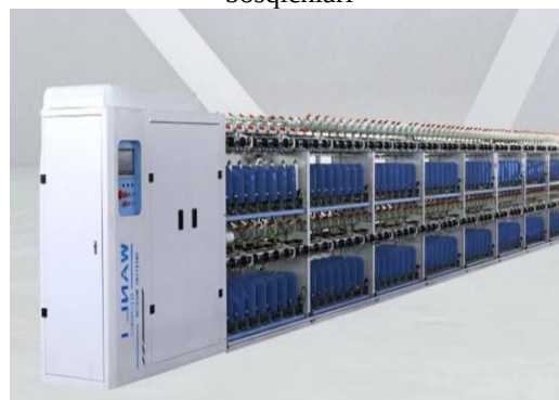
4-rasm. Air-Jet (havo reaktiv) yigirish texnologiyasi
