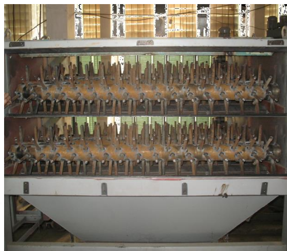
1-rasm. Paxta tozalash agregati uchun yangi titib-ta'minlagichni sxemasi (chapda), tayyorlangan tajriba varianti (o'ngda).
