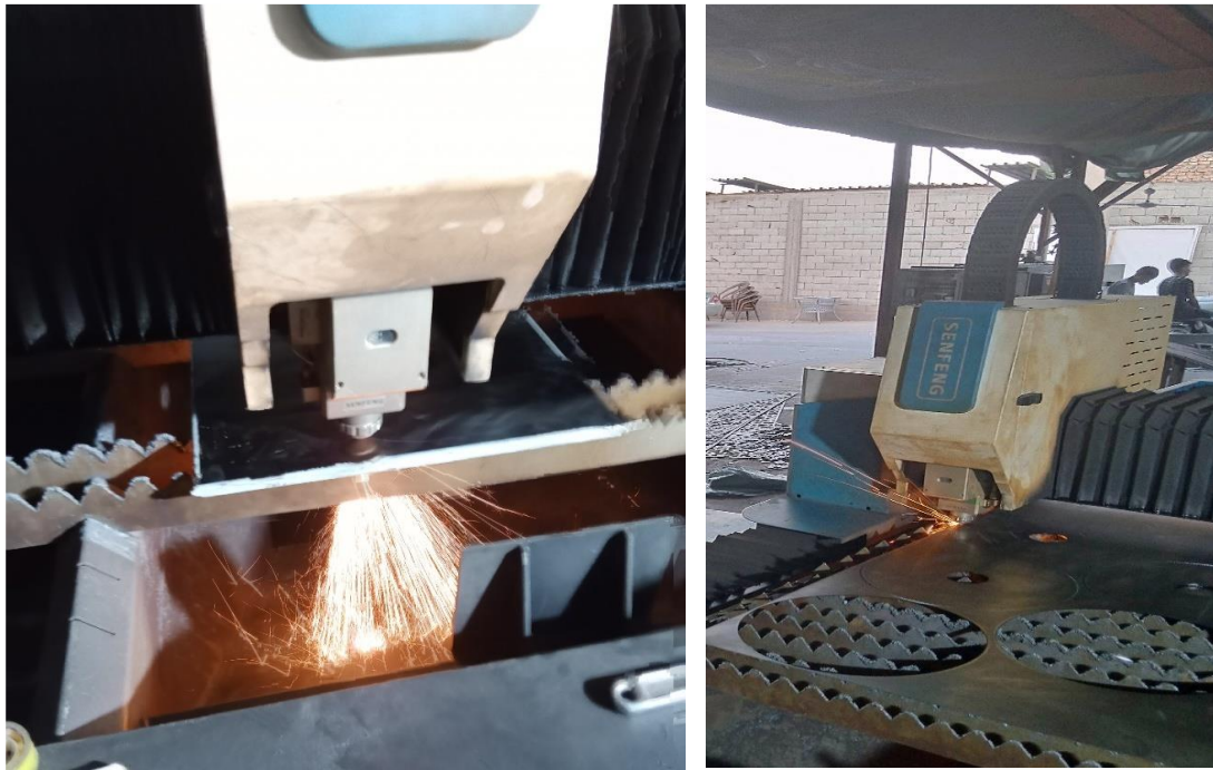
4-rasm. Solid CAM dasturi yordamida yangi tish profilni arra ishlab chiqarish.
