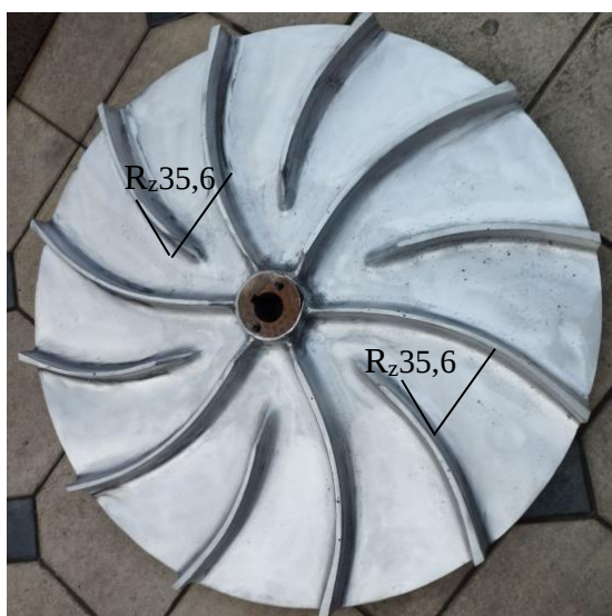
3-rasm. P100 jilvir qog'ozida ishchi yuzasi jilvirlangan parrakli disk ko'rinishi
