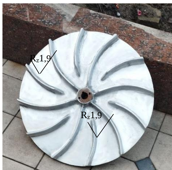
4-rasm. P1000 jilvir qog'ozida ishchi yuzasi jilvirlangan parrakli disk ko'rinishi
