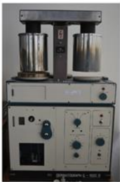
1-rasm. Vengriyaning "MOM" firmasi "DERIVATOGRAPH" termoanalitik qurilmasi va uning sxematik ko'rinishi.
