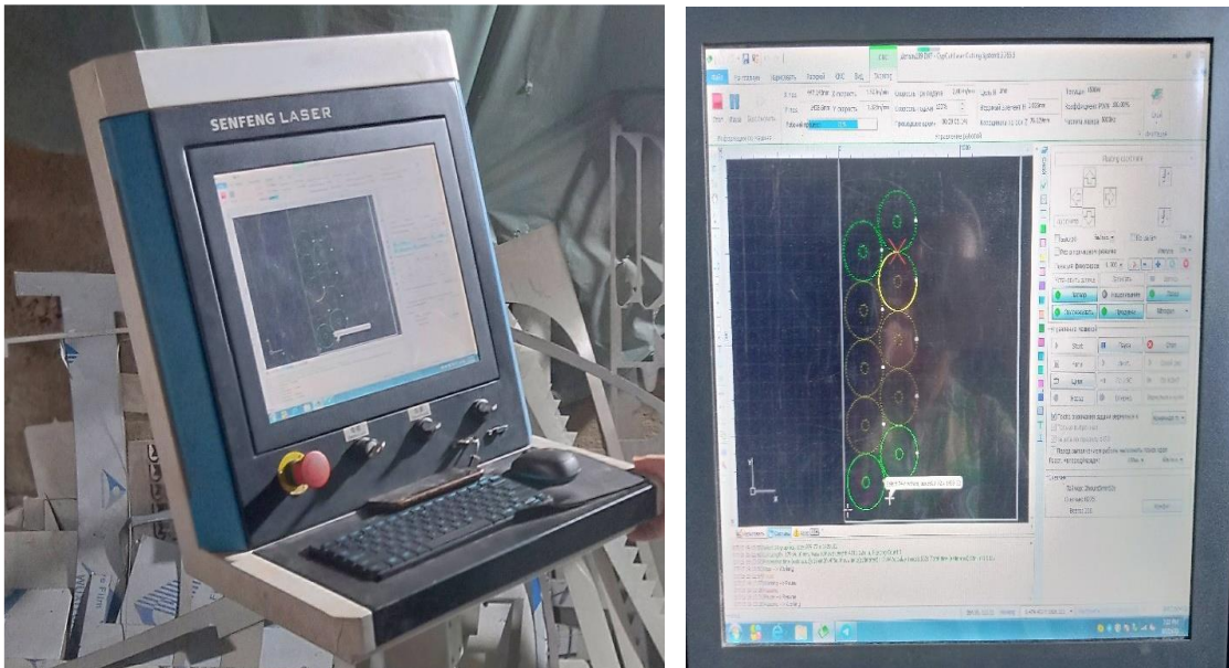
5a-rasm. Solid CAM dasturi uchun boshqaruv pulti
