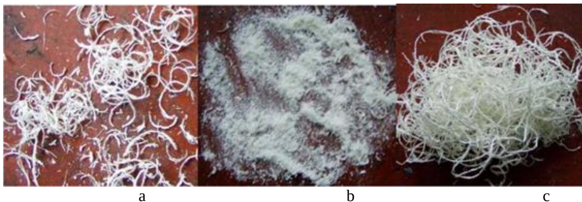
Figure 4. Classification of chips produced in machining fiberglass: (a) discrete, (b) dusty, (c) continuous.
