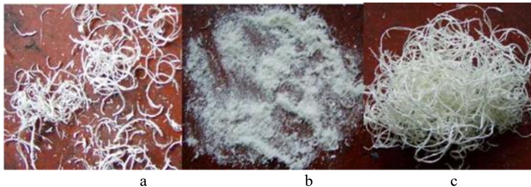
Figure 4 - Types of chips during fiberglass processing:
