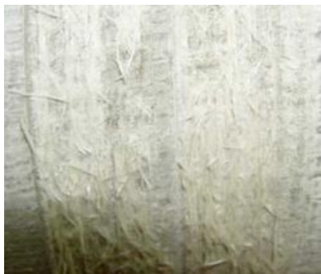
Figure 1. Defect of the treated surface in the form of fraying, which occurs when cutting the fibers.
