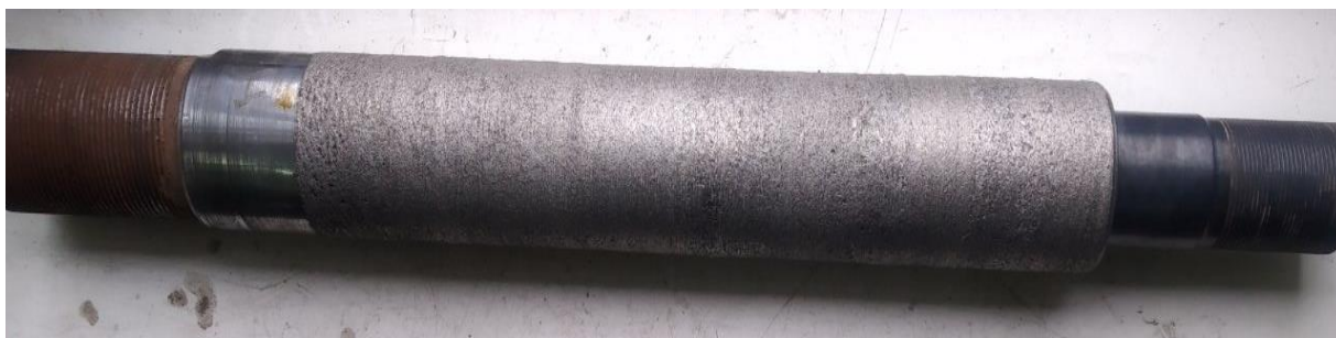
1-rasm. (80%FeQ8%Ni) Q10%SiC Q2%WC bilan qoplama qoplangan val ko‘rinishi
